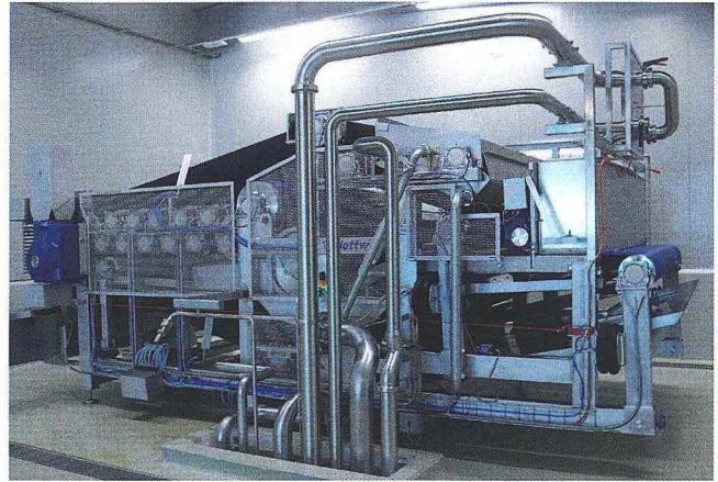
Flottweg belt presses form the central unit for juice extraction after washing, presorting and crushing the apples.
