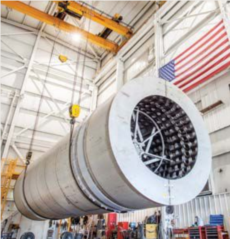
ICM’s energy-efficient rotary dryer used for drying DDGs. Photo Credit: ICM, Inc.
