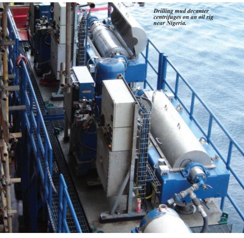
By using decanters at various bore holes, it was possible to partially or even completely forego having to transport the recovered flushing fluids. Only the solids in the centrifuge cake needed to be transported to the mud pit with the remaining flushing fluid.
