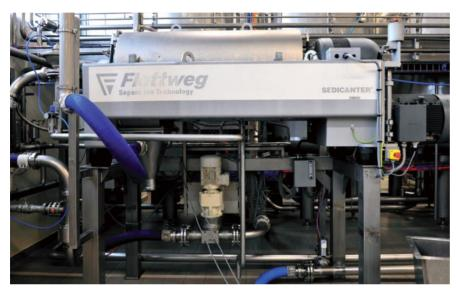
$\label{prop:combines} \mbox{Hygenic Sedicanter} \mbox{\o combines the advantages of a separator and a decanter.}$
