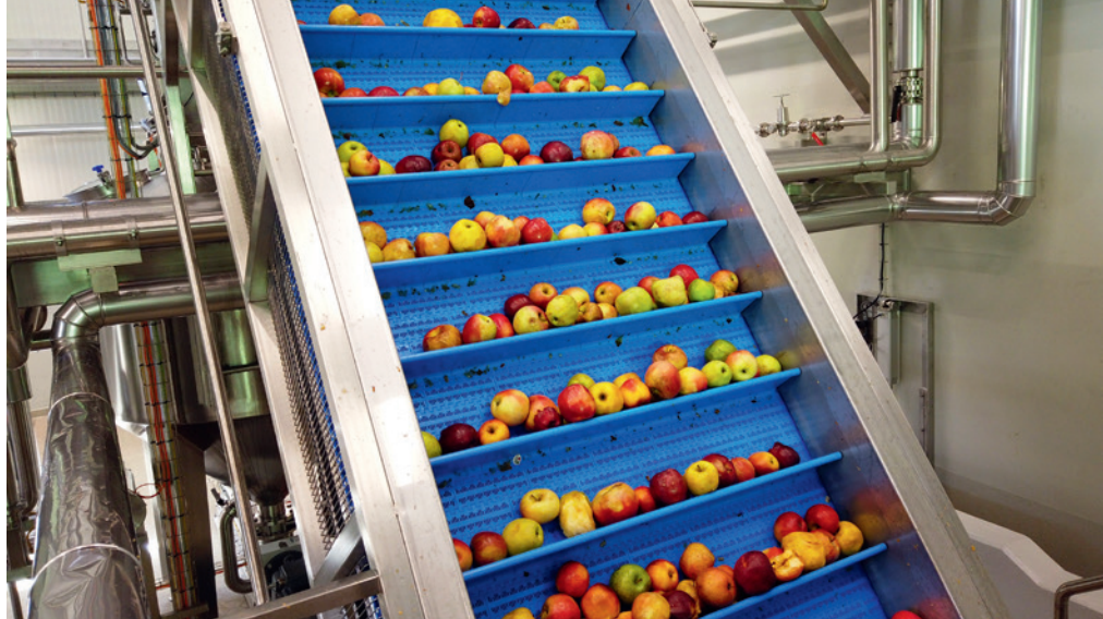
The apples are first washed, pre-sorted and crushed before juice is extracted from them.
