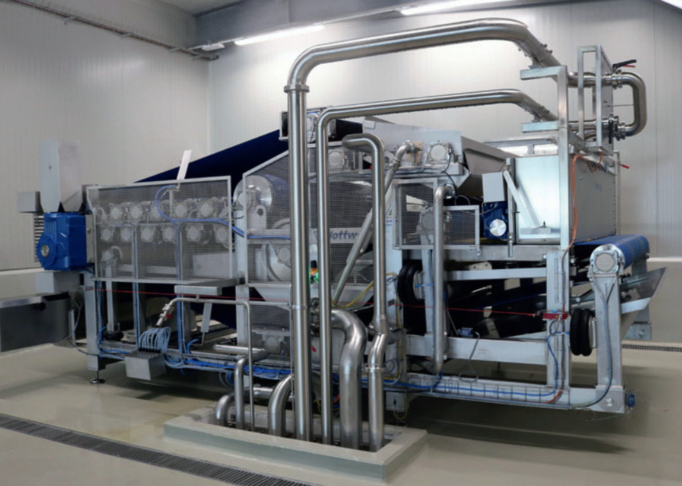
Flottweg belt presses form the central unit for juice extraction after washing, presorting and crushing the apples.
