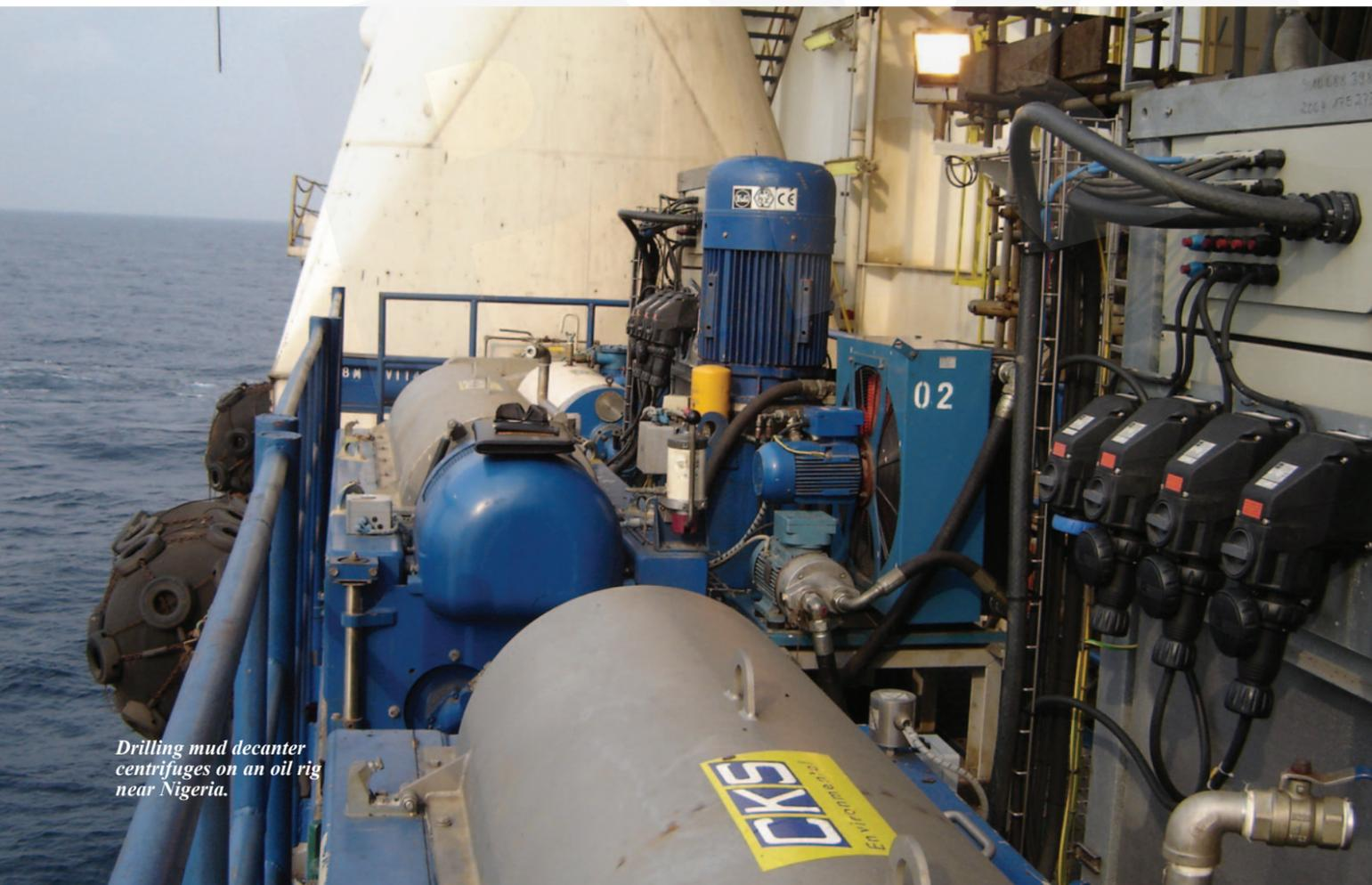
Drilling mud decanter centrifuges on an oil rig near Nigeria.
