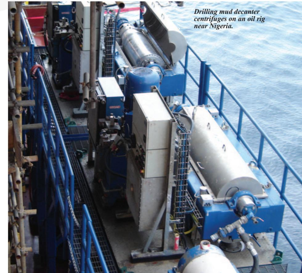
Drilling mud decanter centrifuges on an oil rig near Nigeria.
