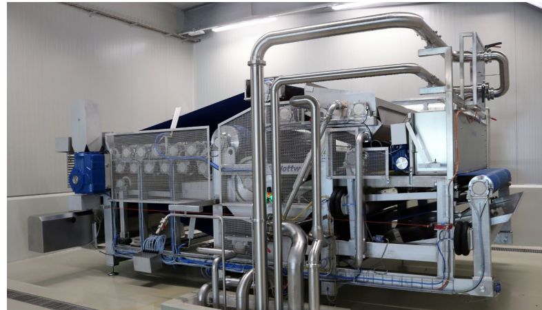
Flottweg belt presses form the central unit for juice extraction.
