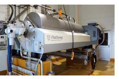
Flottweg industrial centrifuges and belt presses extract starch, fiber and protein from potatoes.
