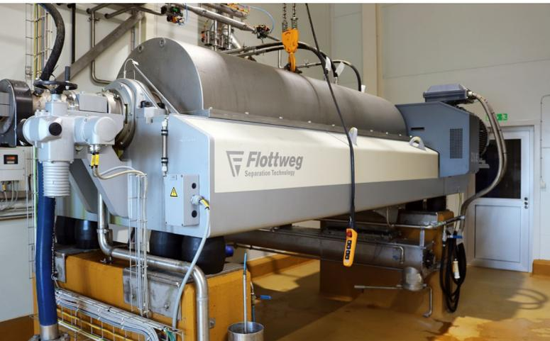
Flottweg industrial centrifuges and belt presses extract starch, fiber and protein from potatoes.
