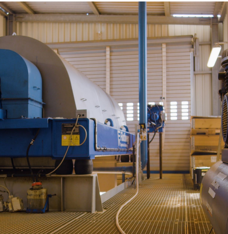
The Z92 decanter centrifuge from Flottweg processes up to 15 tons of the material per hour.
