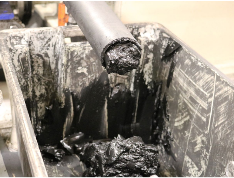
The de-hydrated sludge is temporarily stored in small containers and is then disposed of properly on the mainland.
