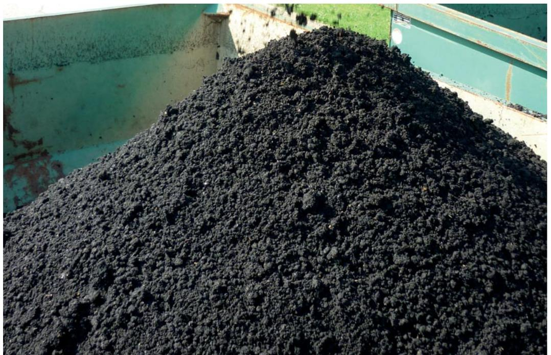
Particularly dry solids after being processed using a Flottweg Decanter Centrifuge
