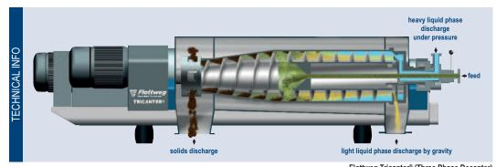
Flottweg Tricanter<sup>®</sup> (Three Phase Decanter) Discharge of the centrate: heavy liquid phase under pressure, light phase by gravity
