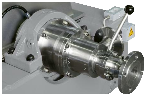
Feed and discharge devices with control lever for the adjustable impeller of the Flottweg Tricanter®
