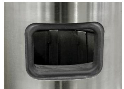
Cake discharge port protected with replaceable bushings
