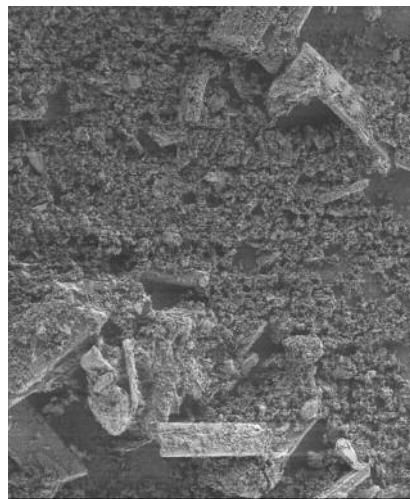
Keep a close eye on your product quality – Zinc sludge SEM analysis (Scanning Electron Microscope)
