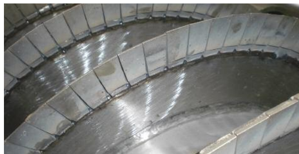
Protection of the scroll with hard metal tiles
