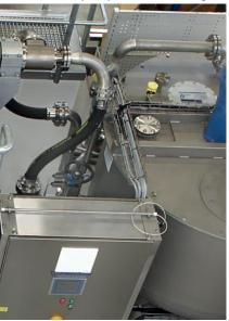
FLOTTWEG SORTICANTER® system From the left: SORTICANTER® with solids discharge, heavy phase, light phase, mixing tank and dosage system
