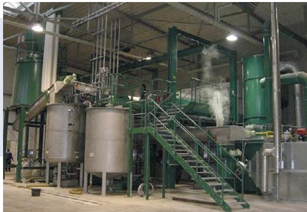
FLOTTWEG SORTICANTER® system for the recovery of polyolefins from mixed plastics at a German company
