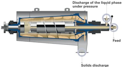
Soft and flowable solids like proteins, pentosan, and so on are hard to process using a standard decanter. Only the patented Flottweg Sedicanter® can provide an optimum result. Even under changing feed conditions, it gets the best separation results thanks to its adjustable impeller.
