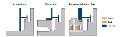
Flottweg Centrifuges adapted to operate in closed-loop systems
