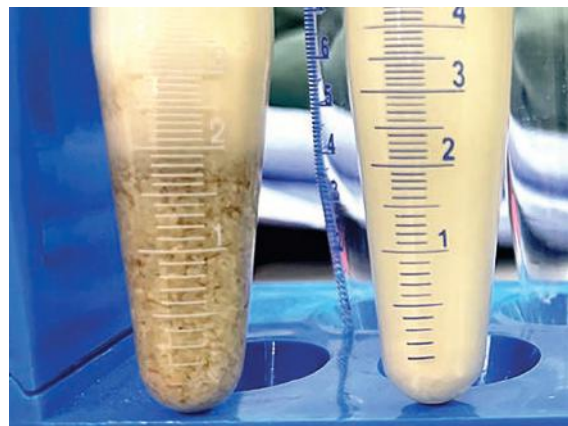
Oat milk before and after the centrifuge. Best product quality thanks to optimum separation.
