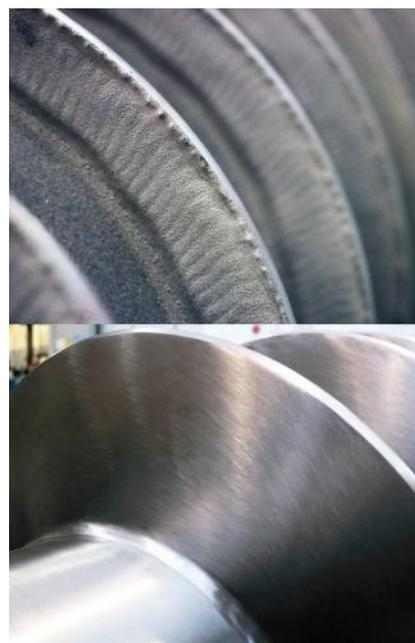
The surfaces of the hygienic scroll that come into contact with food are a maximum of 0.8 µm, depending on the process requirement.
